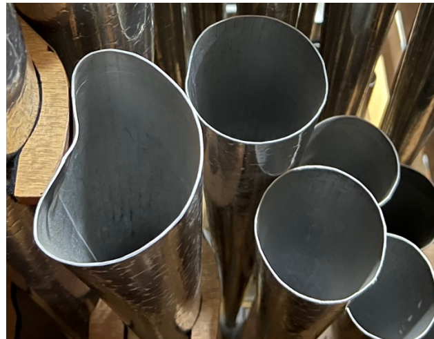
This pipe's resonator width was not considered in the construction, causing it to be cramped by the wooden brace next to it.
